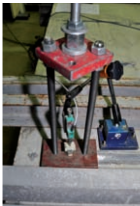
Test setup for cyclic pull out tests
